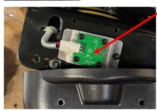
**3:** Note the marking on PCB showing north on magnet towards player side of controller
