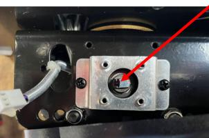
**4:** Black mark on magnet denotes the north pole of the magnet. The black mark should be towards the player side of the controller as shown.
